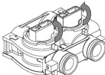
To put the Iron Boss system in bypass position, turn knobs counter-clockwise as shown in picture above.
